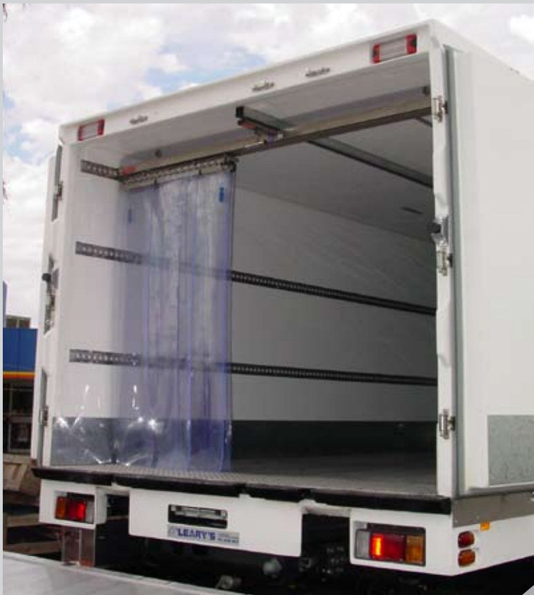
Gliding truck system with an optional triple sliding tracks allows most of the truck body to be opened
