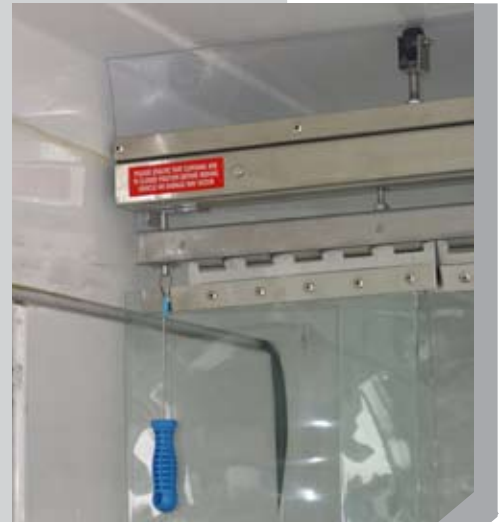
Pull handle latch allows the curtain to slide sideways or be locked
